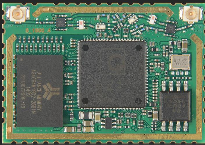
Lima is a QCA-4531/QCA-9531 chipset based module with a 650 MHz CPU and 802.11N 2x2 (MIMO) radio. Module is available in two temperature ranges: commercial\* (Lima) and industrial\*\* (Lima-I).
